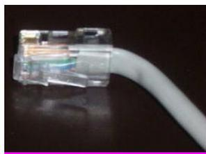
Figura ~~60:61~~ – Connettore maschio RJ45
