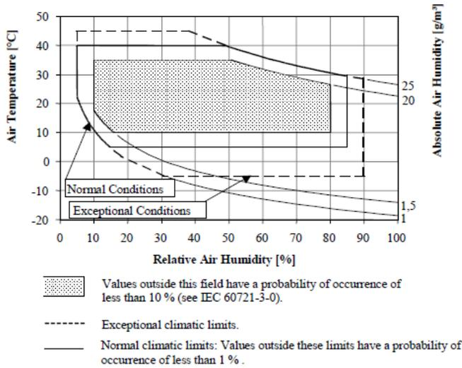
NOTE: Exceptional conditions may occur following the failure of the temperature controlling system. This is described as 3.1E in the tables but it should be noted that there is no separate class 3.1E.
